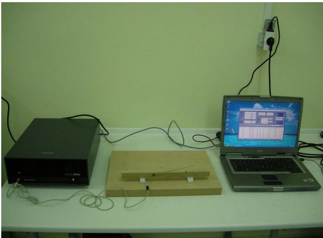
GRINDOSONIC Mk5 device for non-destructive MOE measurements of wood
