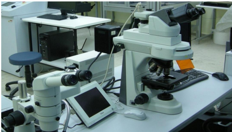
Research microscope ECLIPSE 50i with a digital camera & relative software, and Stereoscope NIKON SM2 800 equipped with photographic digital system
