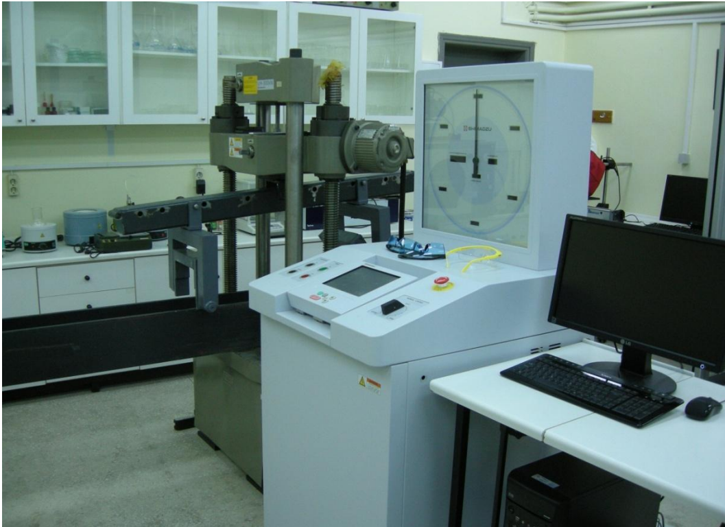
Testing machine SHIMADJU UH-300 kNI for mechanical properties of wood materials
